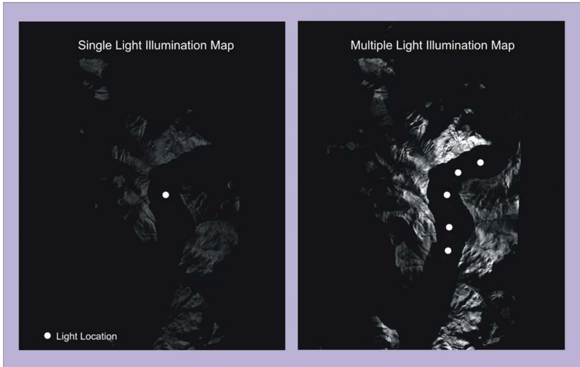
Figure 20 Examples of single light at LCP 120 (left image) and multiple light (right image) cumulative illumination maps (Howe Sound project); Lights are set at the LCPs shown in Fig. 18.
