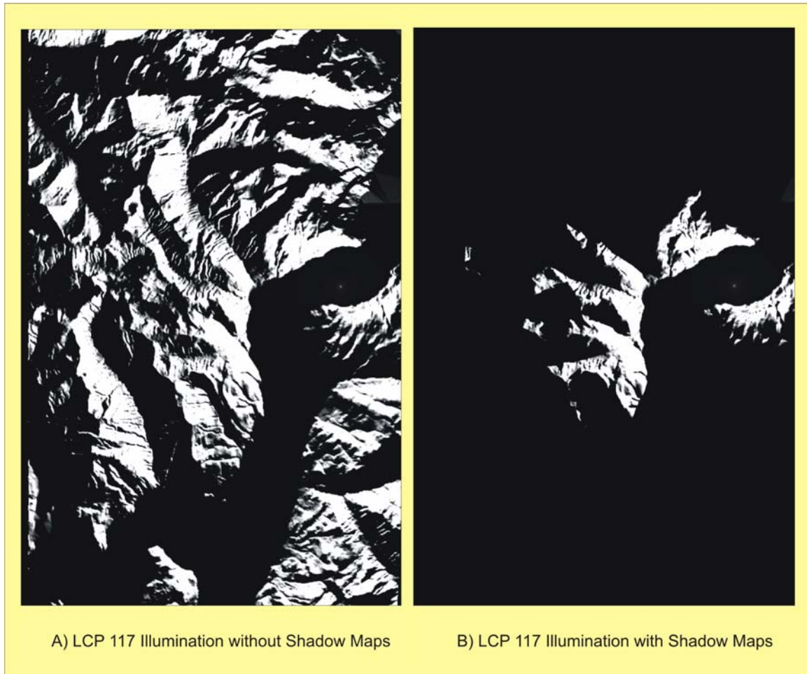
Figure 19 Comparison of terrain illumination in VNS: A) without shadow mapping (an erroneous illumination map); B) with shadow mapping (a correct illumination map).
